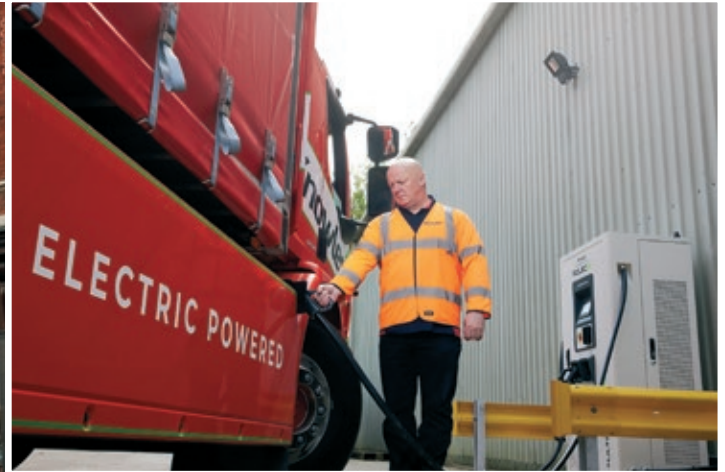
Knowles Transport has invested in a 19-tonne Volvo FE Electric and a 150kWh supercharger, which charges the truck in two hours
