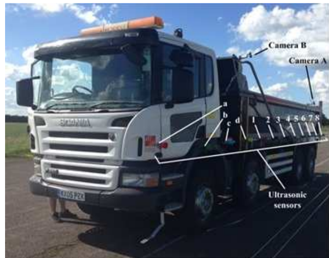
Figure 2. Camera and ultrasonic setup
