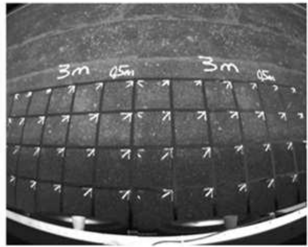
Figure 9. Calibration grid processed to cover the entire image
