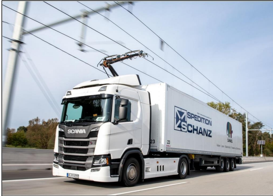
Figure 5.1: Photograph of the catenary ERS demonstrator in Germany.
