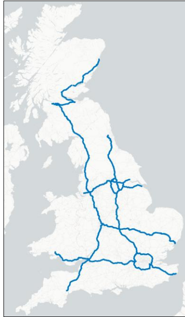
Figure 1: An ERS network of 5,500 single lane-km, supplemented by up to 2,100 static charging stations, would support the UK Logistics industry without requiring any significant changes to current operational practice.
